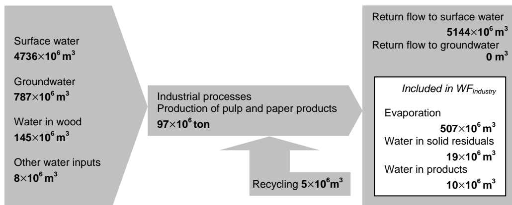
Figure 2. Water flows in the paper and pulp industry in the USA (NCASI, 2009).
